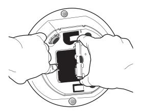
Figure 7. Spectra III/Spectra IV Back Box Interconnect Door
